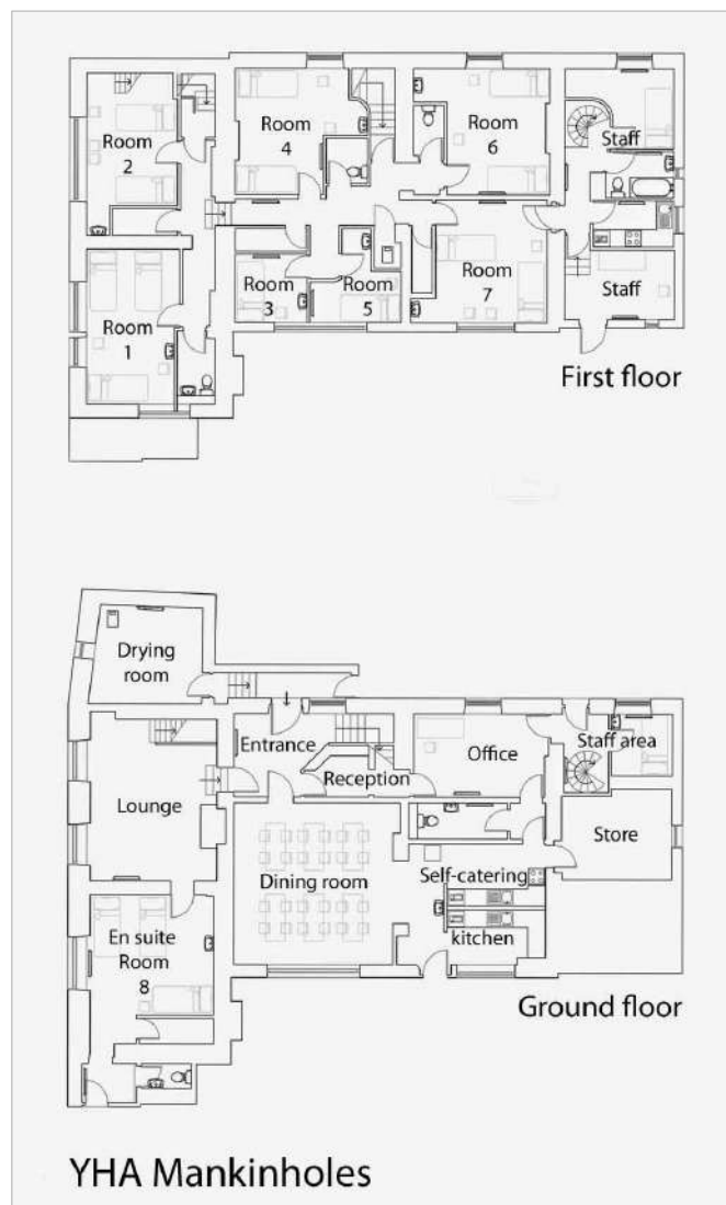
This floorplan of YHA Mankinholes dates from 2016, initially as a CAD drawing but is here redrawn and simplified by the author. It represents the general layout of the hostel from the reorganisation and modernisation of 2000 through to the present time. Bed numbers: Rooms 1 and 8 – 6 beds; Rooms 2, 4, 6 and 7 – 4 beds; Rooms 3 and 5 – 2 beds
